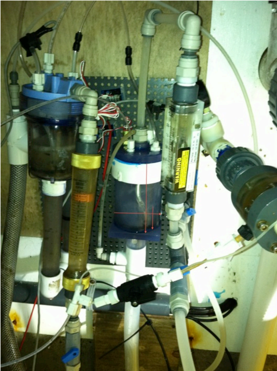
Appendix J. Image of shower-type equilibrator of PC 2 measurements.
