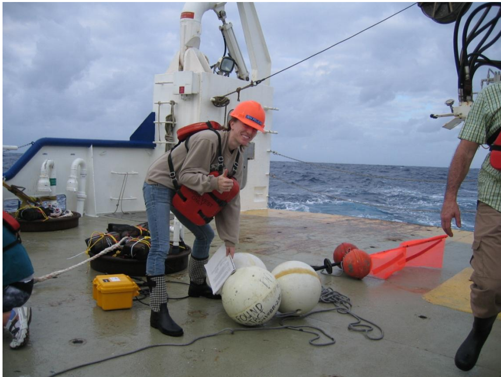
Triple plastic trawl floats with attached spar floats and flag deployed on the Brine Pool Mooring.
