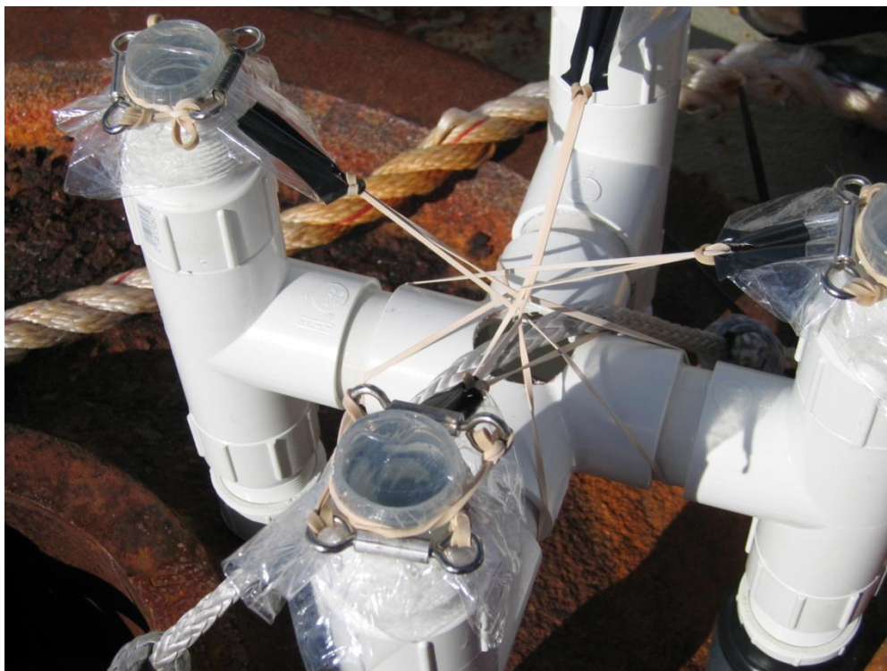
Larval tube traps showing details of the magnesium fusible link release system. Traps were filled with saturated DMSO/NaCl solution.
