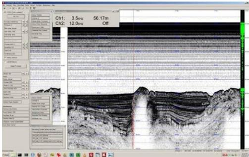
Screen shot from our sub bottom profiler of a pingo-like feature. This instrument interprets the first 100+ meters of sediment below the ocean floor. The layered sediments are our targets (Screen Shot by Woody Sutherland, SIO)
