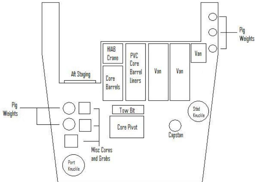
**Figure 1-4.** Jumbo Piston Core (13-02) Fantail storage layout
