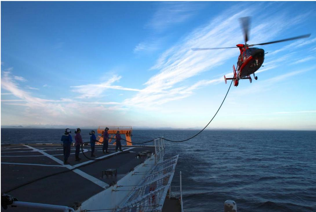
Figure 1-2. HIFR evolution with CG-6518 in the Eastern Bank during Shakedown
