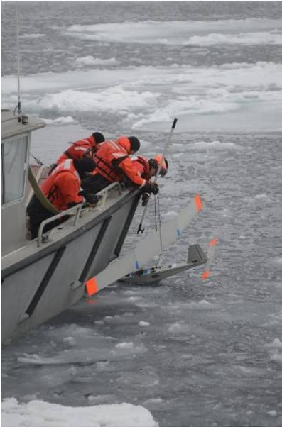
**Figure I-31.** The sUAS is recovered from brash ice by the ASB
