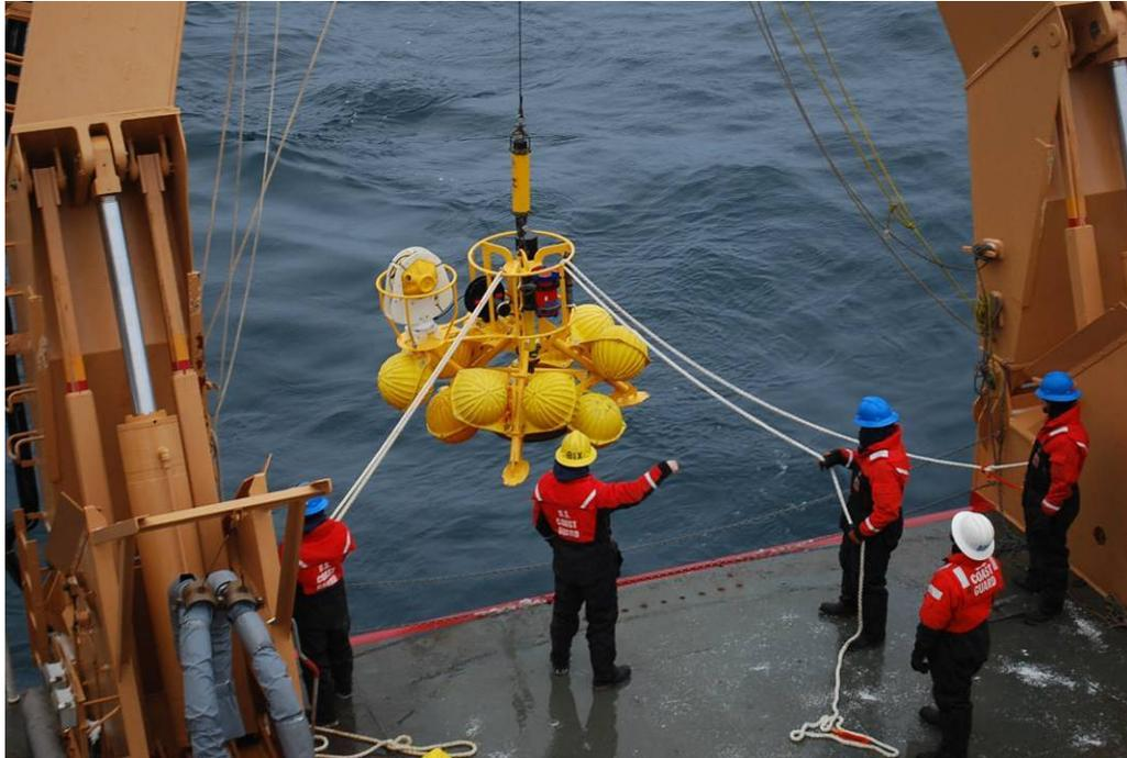
Figure 1-36. Deck crew deploys the CT1 “Tripod” Mooring
