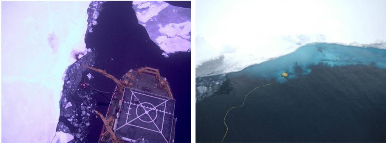
**Figure 1-30.** (Left – photo taken by sUAS) HEALY deploys the skimmer to clear mock oil from near an ice floe
