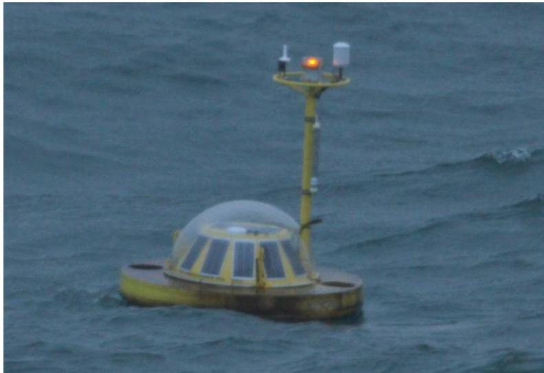
**Figure 1-42.** Wave Rider Buoy
