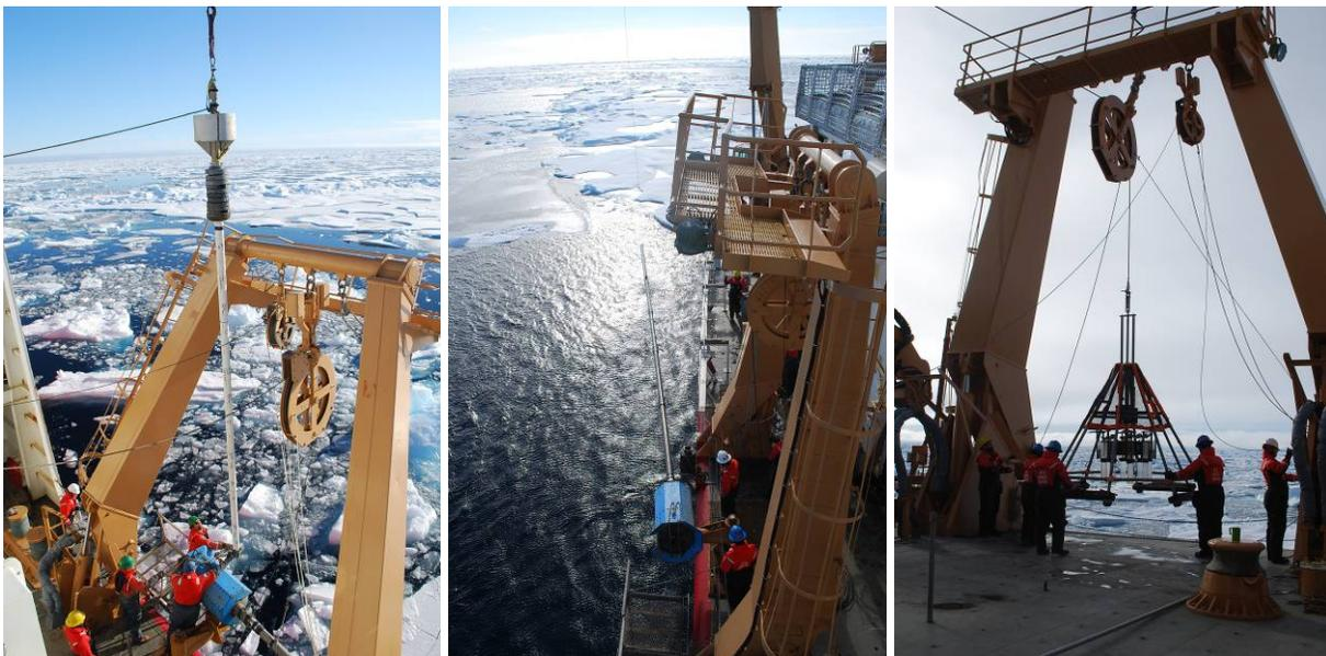
Figure 1-27. Gravity Core, Jumbo Piston Core, Multicore (from left to right)
