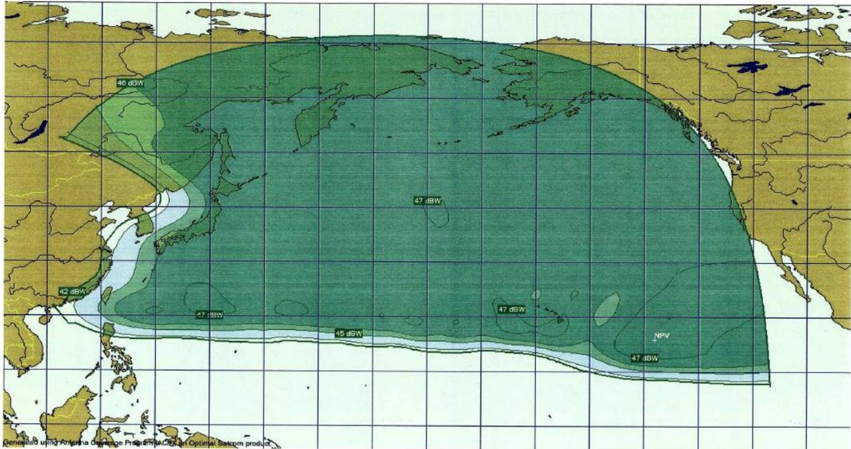
Figure 2-2. INMARSAT Ku-Band E-172A North Pacific Beam Coverage
