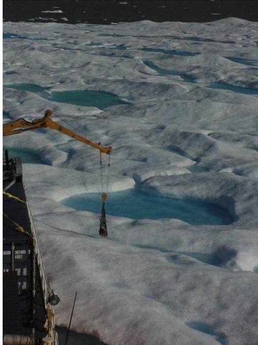
Figure 1-25. Drifter Buoy deployed on MYHF
