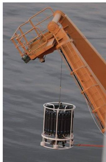
CTD being deployed from the starboard A-frame (Photo by BMCM Sullivan)
