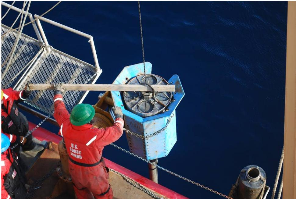
viii. Install the two safety pins into the pivot stand to keep barrel from rotating and falling out when horizontal.<sup>1</sup>
