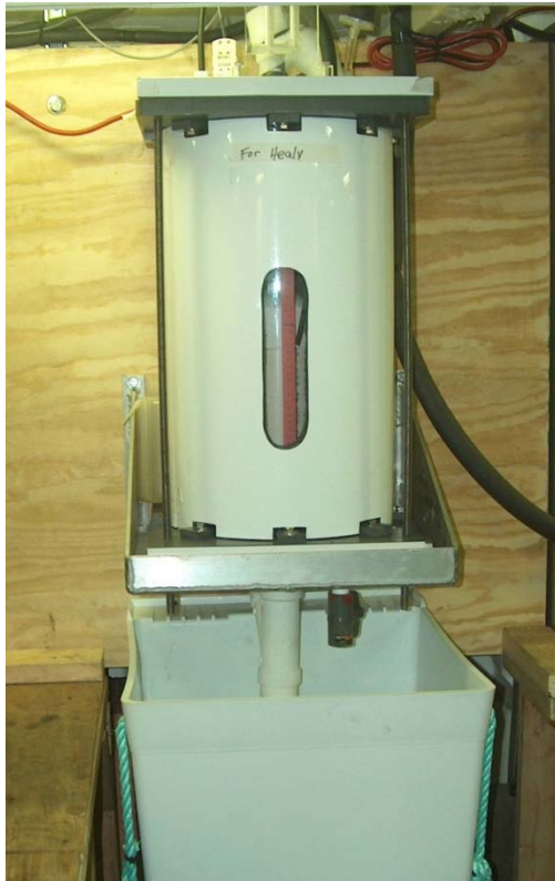
Figure 7: Equilibrator as installed over the sink in the Wet lab.
