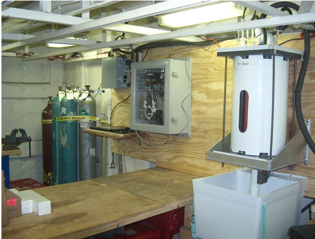
Figure 2: View of pCO 2 system from a forward and port side vantage point (looking to the starboard and aft. Calibration gases and Nitrogen cylinders are farthest to the starboard side of the lab, Air sample pumps are located in the small enclosure that is mounted above the small shelf that holds the laptop computer. The analyzer unit is in the clear fronted fiberglass enclosure and finally the air-sea water equilibrator is mounted on its aluminum shelf above the plastic sink.
