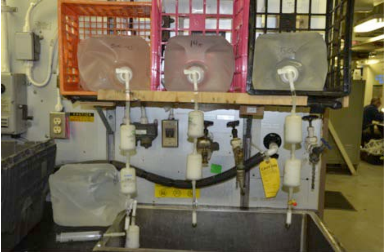
Figure E6. Water from different depths from CTD were collected and filtered for microbiological analysis on-shore.
