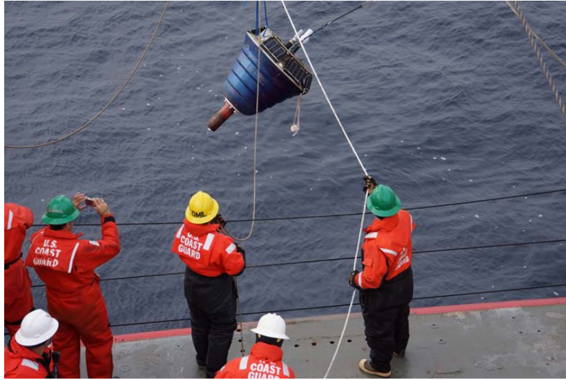
Figure B4 - Deployment of USNA IceGoat-1 seasonal buoy with Glass Planet monkey's fist from the Healy fantail using the A-frame crane on 22 September
