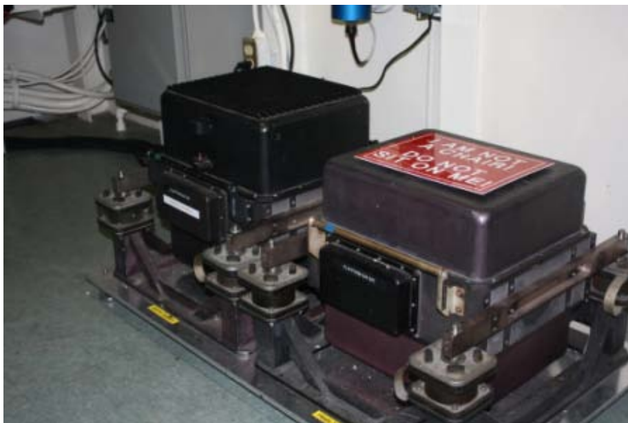
Figure A1 - Dual BGM-3 gravimeters installed on board USCGC Healy
