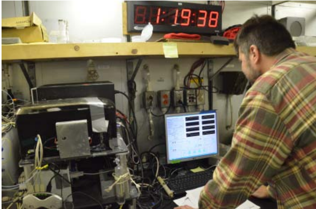
Figure E8. Multiparameter Inorganic Carbon Analyzer, which collected DIC, pH and pCO 2 data for part of the cruise.
