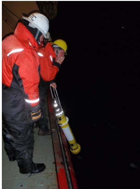
Figure B5 - Deployment of ARGO profiler on 22 September
