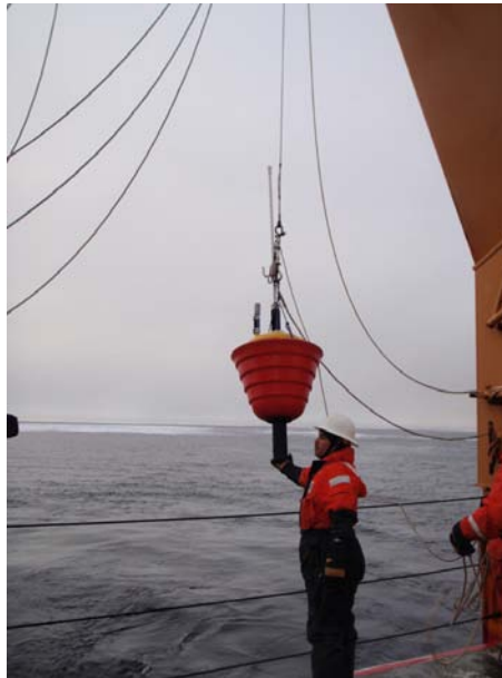
Figure B2 - Deployment of AXIB 018 seasonal buoy from the Healy fantail using the A-frame crane on 30 August 2012
