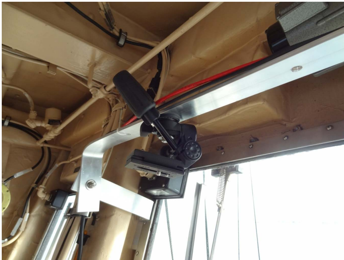
Figure D3: Customs mounts built for the side looking cameras.
