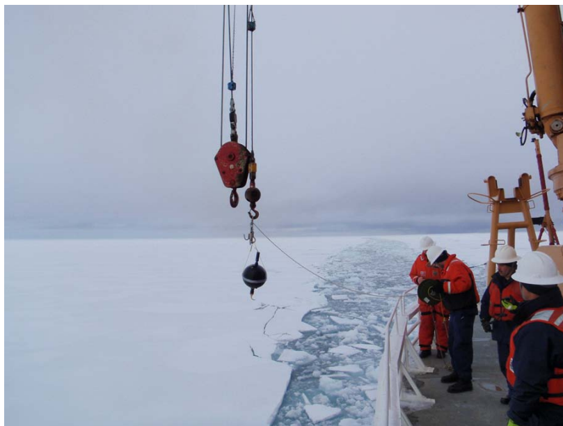
Figure B1 - Deployment of an SVP buoy as an ice beacon on FYI floe on 5
