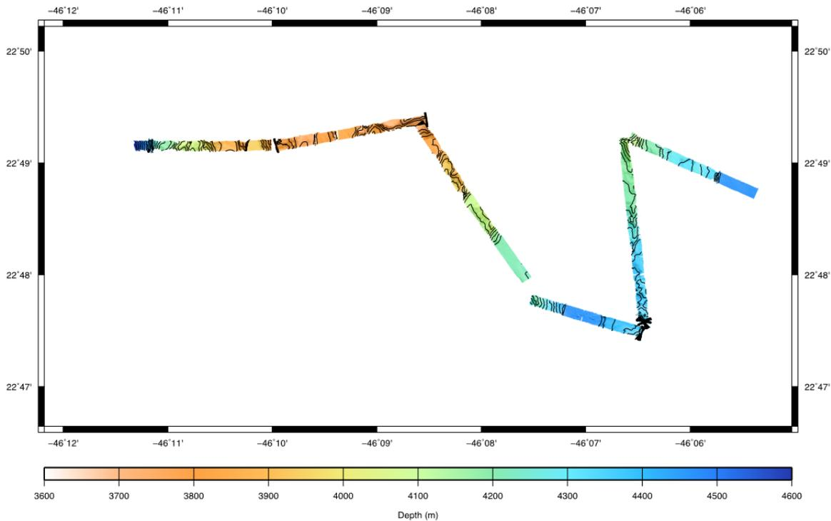
**Fig. 5.24** Jason-based microbathymetry recorded during dive 631
