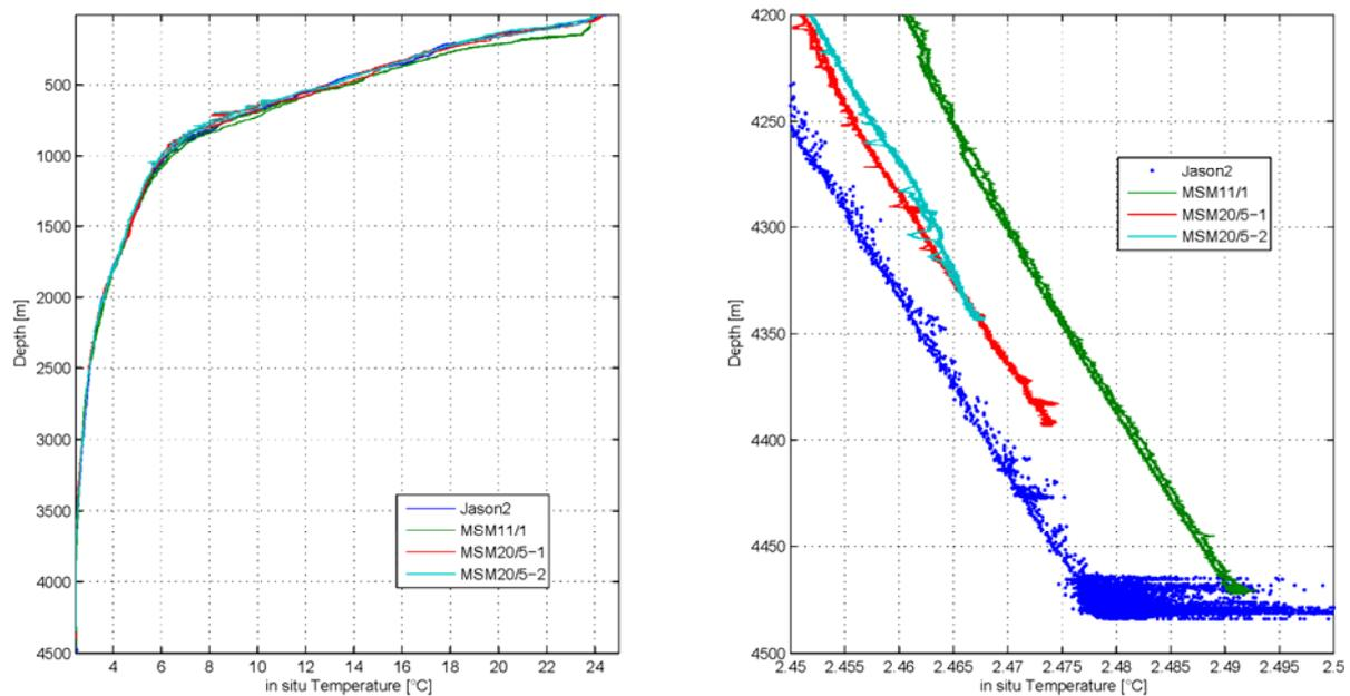
**Fig. 5.2** Comparison of temperature profiles from two CTD casts during MSM20/5, one cast from MSM11/1 and data from the ROV Jason CTD.
