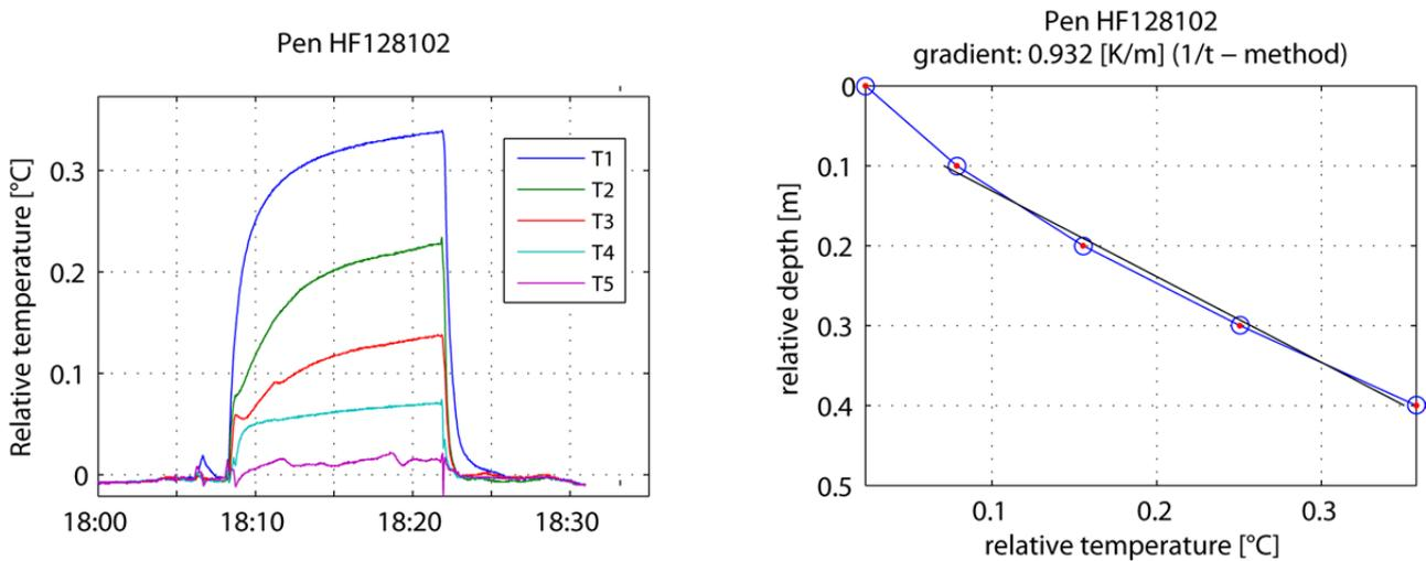
**Fig. 5.23** Example of a very high heat flow measurement with of about 932 mW/m<sup>2</sup>
