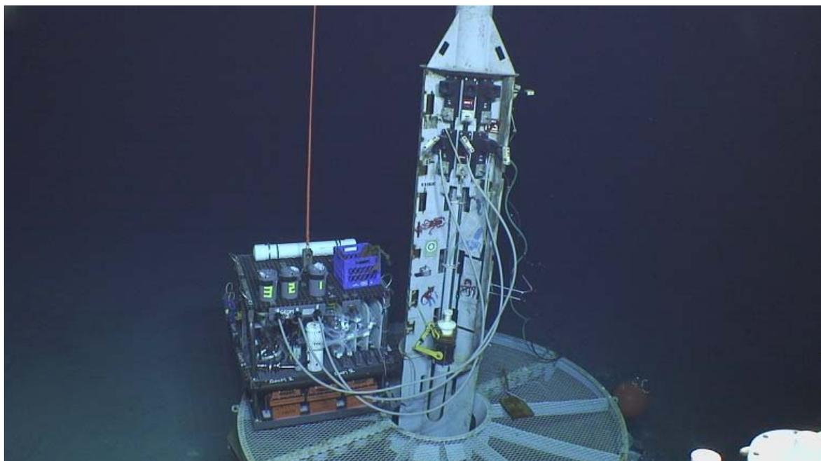
**Fig. 5.12** GeoMICROBE Sled connected to CORK U1383C microbial bay. Three umbilicals connect to three Tefzel fluid delivery lines, which extend to deep (170 m), middle (130m) and shallow (70m) horizon.
