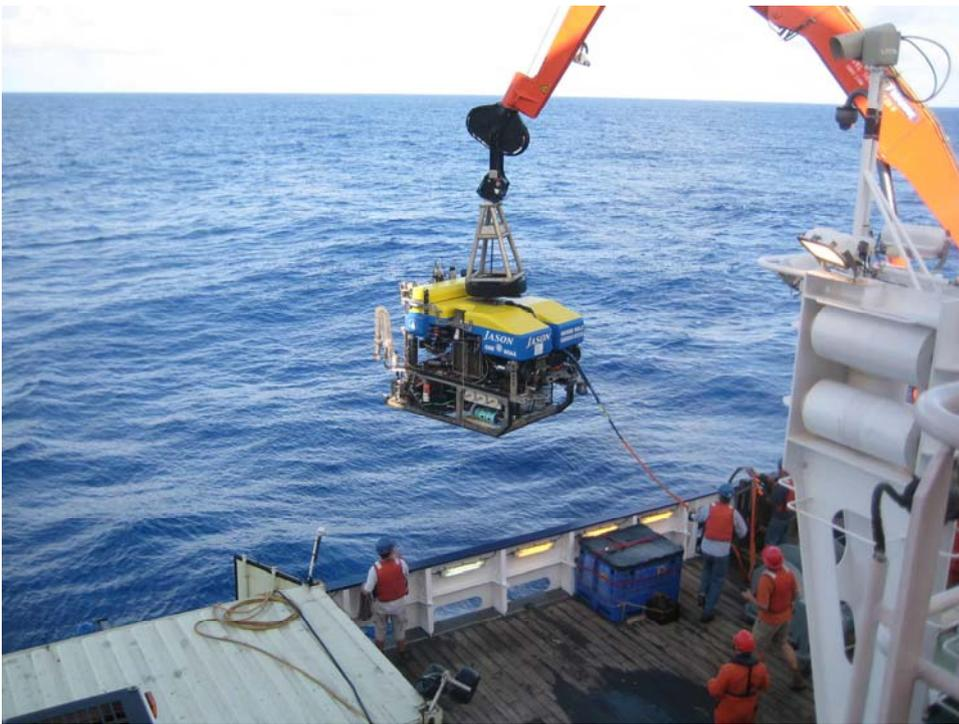
**Fig. 5.3** ROV Jason is launched using the starboard aft crane on the main deck
