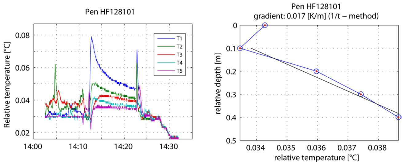
**Fig. 5.22** Example of a heatflow measurement with a low heatflow of about 17 mW/m<sup>2</sup>
