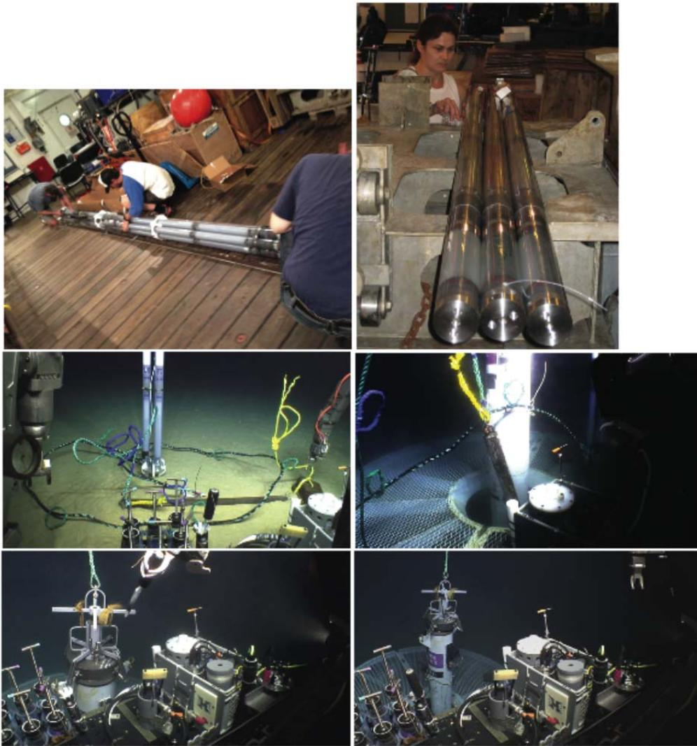
**Fig. 5.8** Preparation and deployment of the CORK lite instrument string in Hole U1382A
