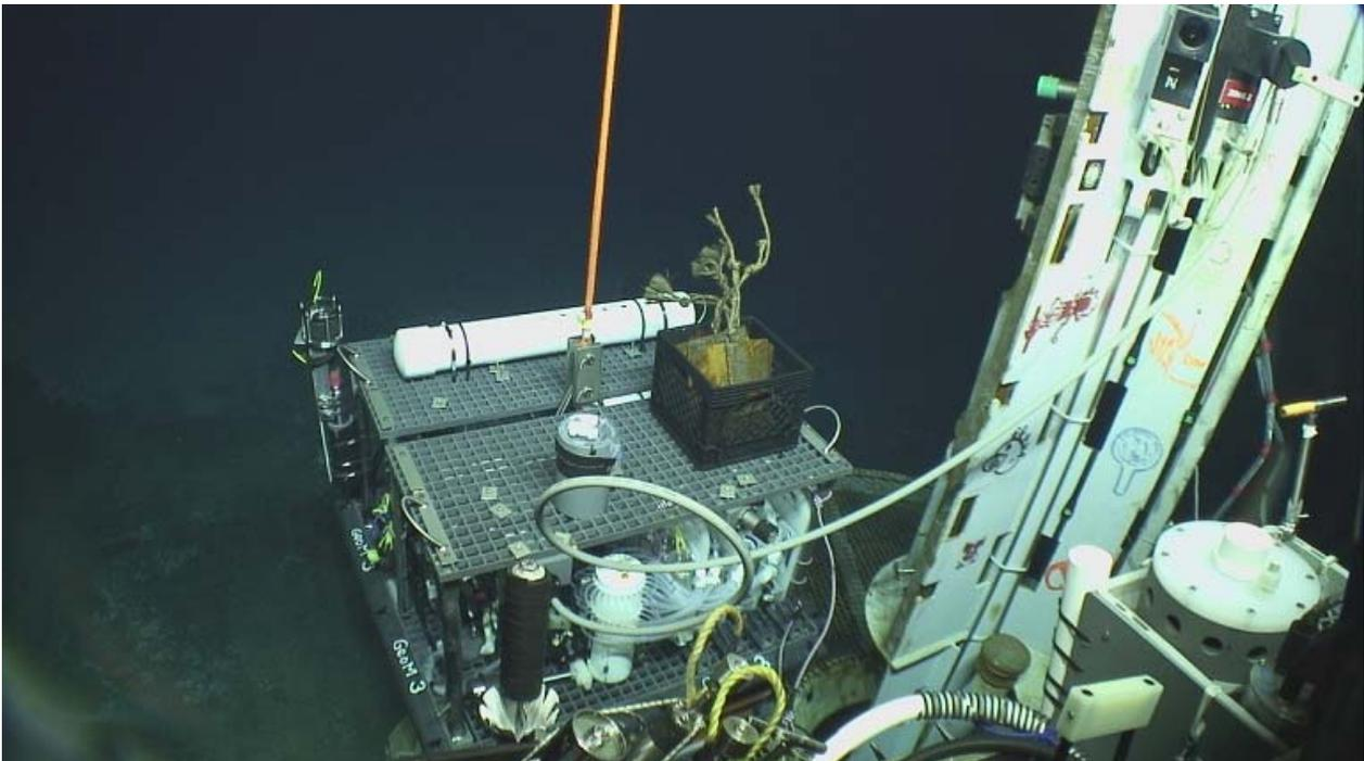
**Fig. 5.11** GeoMICROBE Sled connected to CORK U1382A microbial bay; Tefzel fluid delivery line.
