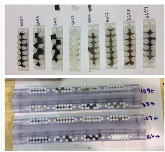
**Fig. 5.7** Incubation substrates mounted in the FLOCS units in Hole U1382A
