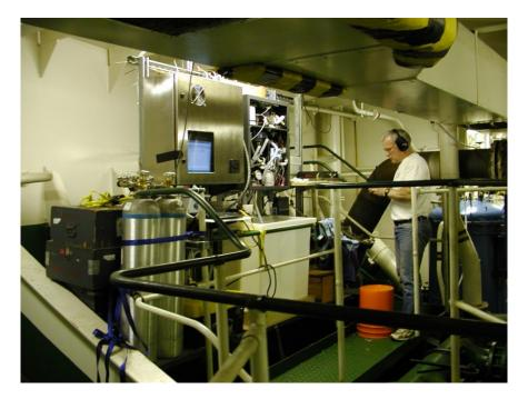
In addition to CO<sub>2</sub> values, the system collects the following data: Surface seawater temperature at the seawater intake Seawater temperature from the equilibrator Conductivity and salinity from a Seabird TSG mounted next to the pCO<sub>2</sub> system Barometric pressure in the Licor, and in the equilibrator Latitude and longitude from a GPS mounted near the bridge Sea surface temperature, salinity, and barometric pressure are necessary to calculate partial
