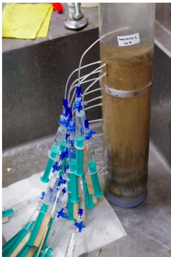
Fig. 1.14. Rhizon pore water sampling from multi-core GeoB15103-3.
