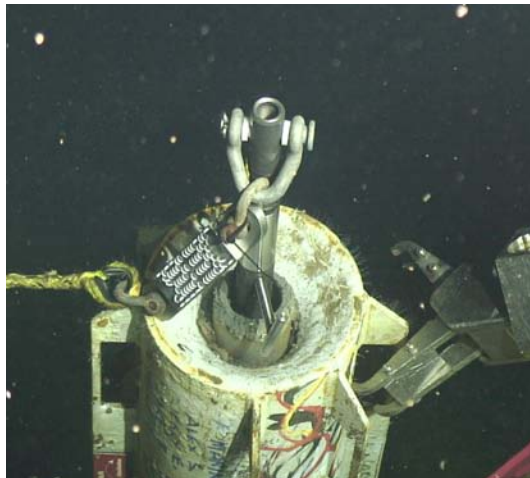
Image of the top of the 1362A wellhead with the GS pulling tool and weak-link in place and the basket prior to the dive.
