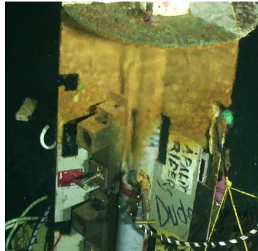
Image of the Alvin basket before launch and the wellhead at 1362A in the MBIO bay. Note the venting water from the flow meter chimney (a 4"-diameter PVC tube) and the microbial material on the wellhead.
