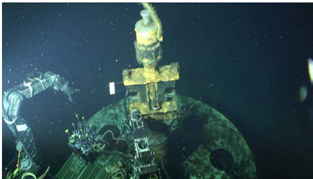
The new logger is connected to wellhead.
