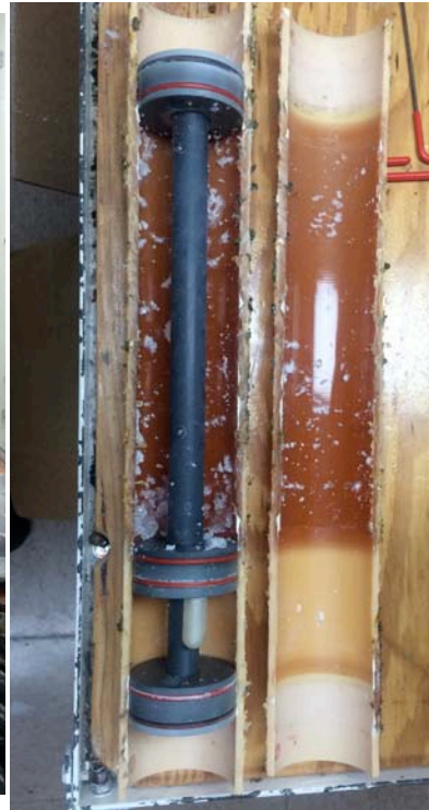
Work on a downhole OsmoSampler (1362A). We recovered standard, copper, acid-addition, enrichment, and BOSS OsmoSamplers. A close-up of one of the downhole pumps from 1362A.
