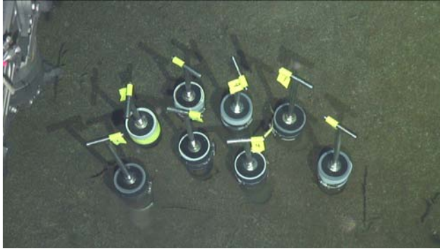
Push Core arrangement on the seafloor
